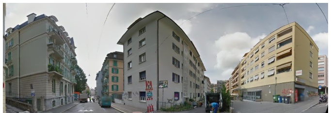
Figure 1. The panoramic output has a much larger field of view and allows much more information to be captured, however in 2d the façade of the building is distorted and might affect the opening to façade ratio. Additionally, this higher quality required 50 separate images from the Google Street-view API.
